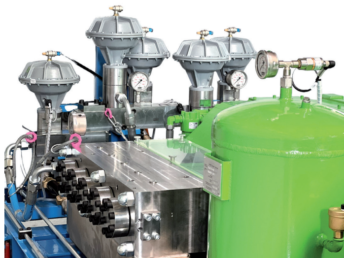
Fig. 1: Valve arrangement of a combined test system
