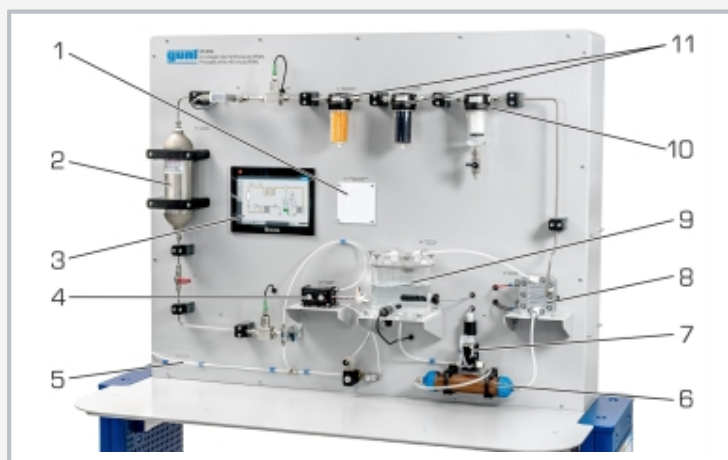
1 halogen lamp as electrical consumer, 2 buffer tank for H 2 , 3 touch screen, 4 PEM fuel cell, 5 H 2 excess: extraction or discharge to the outside, 6 ion exchanger, 7 diaphragm pump, 8 PEM electrolyser, 9 water tank, 10 water separator, 11 drying units
