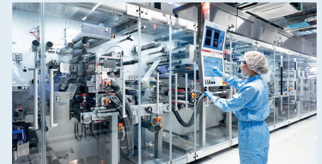
4 Converting machine pre-cuts CCM and subgaskets in several process steps and combines them to form 5-layer MEAs.
