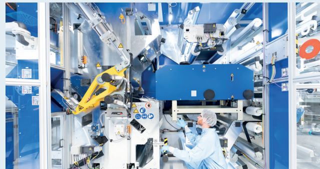
3 R2R transfer machine to transfer anode and cathode catalyst layers from decal films onto the membrane.
