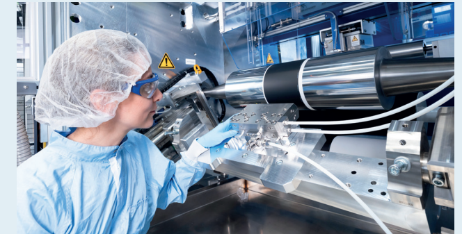
2 Roll-to-roll coating line to apply catalyst layers on decal films or membranes.
