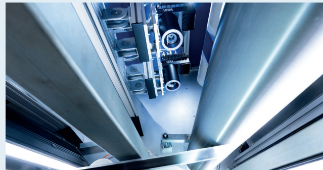
5 In-line quality control using optical line scan cameras.
