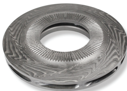
2nd Impeller Design (Failed at 534 m/s)
