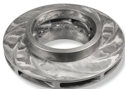
1st Impeller Design (Failed at 500 m/s)
